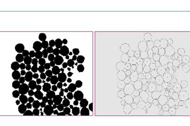
A script was written to automate aggregate size distribution analysis. Phase-contrast captions of aggregates from culture samples were analysed using ImageJ software (image above with aggregates sampled at day 4 of culture in Ambr $^{\mathbb{R}}$ 15. Scale bar 1000  $\mu$ m).
