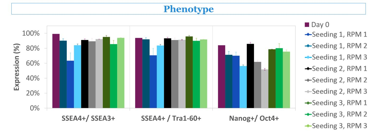
Cell counts and viability were measured after dissociation of aggregates. Higher impeller speeds shows a positive effect on day 1 cell survival but a negative effect on total population doublings and co-expression of NANOG/OCT3/4. Aggregate size of approximately 400 mm is maintained after day 3 at all agitation rates of cultures seeded a Seeding 3. A 75% (v/v) daily medium exchange with two exchanges on day 4 was the medium exchange regime used herein as result from previous investigations.
